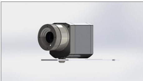
Figure 13: Fully assembled PI camera on mounting plate
